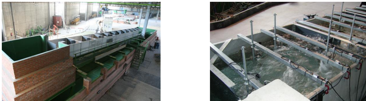
Figure 1. Indoor full-scale vertical slot fishway model used in this study (left) and detail of the network of video cameras which was installed in the model (right).
